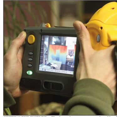
GETTING THE PICTURE— The thermal camera captures the cold and heat distribution of interior walls. Red shows heat, green and blue signal
